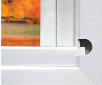
The sill dam wall is mortised into the jamb adding strength and lowering the possibility of leaks that may occur at corner seals.
