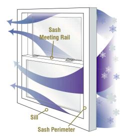
Poorly designed windows don't have the built-in airlocks, weather stripping, and barriers necessary to keep air from forcing its way in. Without these design features, air will push between the sash meeting rails and around the sash perimeter where it meets the frame and sill.
