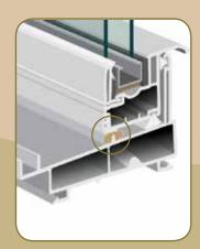
Soft-Seal™ straddle gasket is a closed-cell neoprene cushion-gasket under the sash that straddles the sill rail and helps prevent air and water infiltration.
