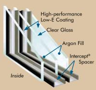
Above values are for a Barrington double-hung window with Ultra Glass, featuring single-strength glass, Intercept Spacer, argon gas, and without grids.
