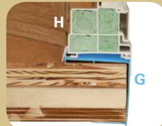
G. Exclusive welded sill pan (highlighted in blue) eliminates water penetration. The unique design provides a built-in weep system and a smooth finish on the exterior surface of the seat board.
