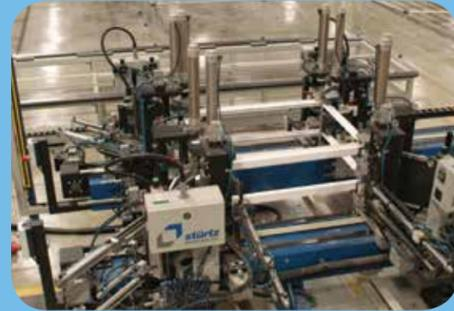
To ensure "perfection" both sashes are welded simultaneously. Prior to welding, sensors determine whether either sash is less than "perfect" ( $\pm 1/32"$ ). If they are not perfect, both sashes are rejected automatically by the equipment.
